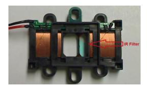
The cut filter is activated during the day to remove IR light, as it may cause <u>color shift/white balance issues</u>, such as the pinkish grey trees and desaturation seen in the image below:
