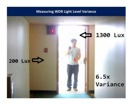
The WDR ratio is  $^{\sim}6.5x$ , with the open doorway at 1300 lux and the adjacent indoor sides at  $^{\sim}200$  lux.
