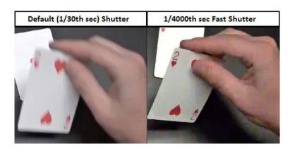
1/4000s shutter speed completely eliminated all traces of motion blur.
