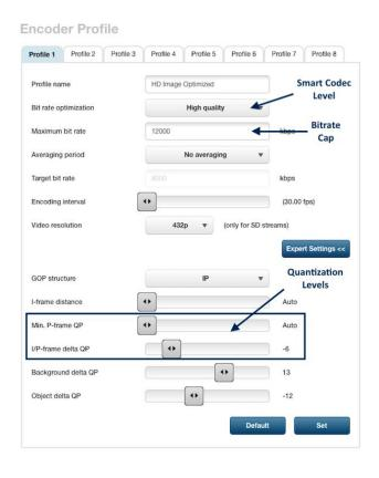
For MBR, simply set the maximum bit rate to what you would like your cap to be. The target bitrate is effectively a minimum bit rate.
