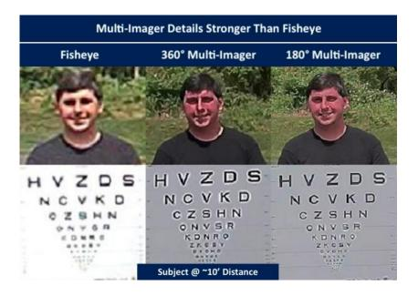
With the subject at ~30' from the cameras, the fisheye panoramic provides no usable details whatsoever, while the 360° multi-imager still provides two legible lines of the chart and some rough subject details. At this distance, the 180° multi-imager still provides recognizable details of the subject.
