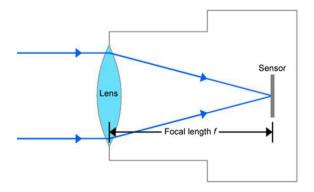
The longer the lens is, the farther it is away from the imager, resulting in a narrower FoV.
