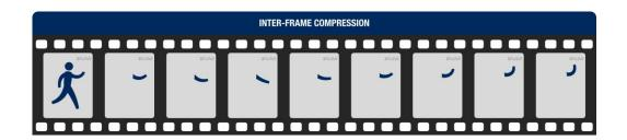
With so much of a given scene remaining static, sending only changes in the scene saves substantial bandwidth/storage. For instance, the same 1080p/30fps stream that might need 40Mb/s with MJPEG, an intra-frame only codec, may only need 4Mb/s with H.264, a codec that uses both.
