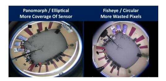
However, we have not found substantial practical differences in our tests, with standard fisheye models performing as well as ImmerVision-based models.
