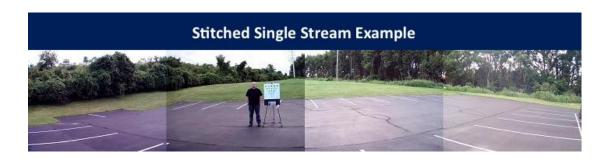
Stitched streams are moderately more usable as they allow the full panorama to be navigated at once, instead of moving from camera to camera. However, when placed in a typical layout with other cameras, they may appear small and/or strange due to their non-standard wide aspect ratio, seen here:
