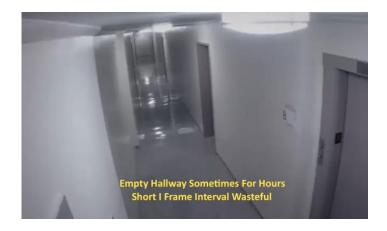
But when the burst of people walk through, I frame interval should be shortened to reduce artifacts and other issues (see <u>Test: H.264 I vs P Frame Impact</u>).
