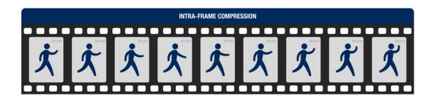
The upside is that this is simple to do computationally and does significantly compress video. For instance, a 1080p/30fps video stream using an intra-frame compression like MJPEG can have its bitrate reduced
