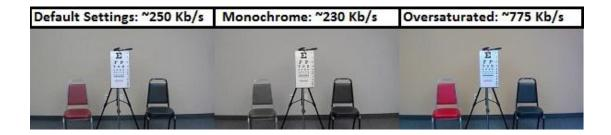
One practical example of a manufacture desaturating their video to 'save' bandwidth is Arecont Bandwidth Savings Mode (which we tested here).
