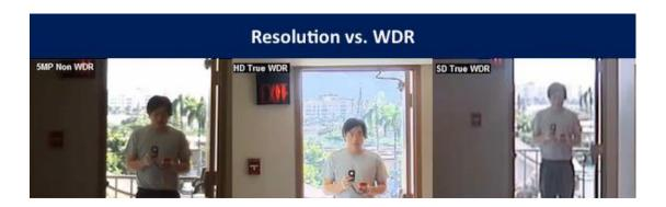
The worst performer is the SD camera, even though it use true WDR. The 5MP non WDR camera beats it simply because it captures more details. Finally, the HD camera with true WDR performs the best.
