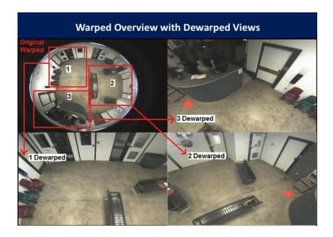
This dewarping is a critical component of fisheye panoramics. Warped video, by itself is practically useless. Manufacturers can dewarp at the camera side, client side or both. The choice of where to dewarp impacts VMS integration and usability greatly.
