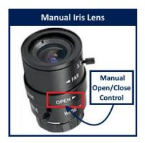
Manual iris lenses allow the iris to be controlled by manually rotating a ring on the lens. Though the iris is controllable from all the way open to all the way closed, manufacturers generally recommend setting manual iris lenses either fully or 90%+ open to maintain low light performance. Manual iris lenses are uncommon but still used in some specialist applications.
