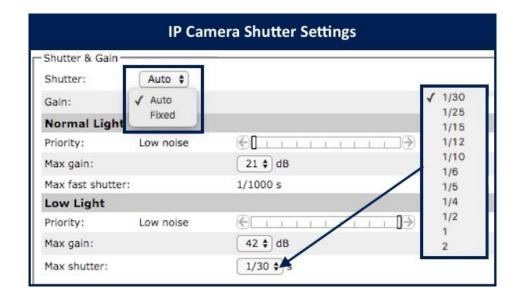
In 2017, nearly all cameras use automatic shutter speed, but manual settings are still used in some specialist applications such as <u>license plate</u> capture / recognition and machine vision.
