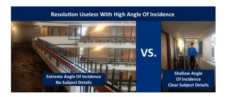
Even if the image on the left had 10x the pixels as the one on the right, the left one is incapable of seeing the full facial details of the subject as he is simply not facing the camera.
