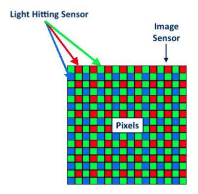
For example, a 1080p resolution camera is commonly described as having 2MP (million pixel) resolution because the sensor used has  $^2$  million pixels on it (technically usually 2,073,600 pixels as that is the product of 1920 horizontal x 1080 vertical pixels). The image of an imager below shows this example:
