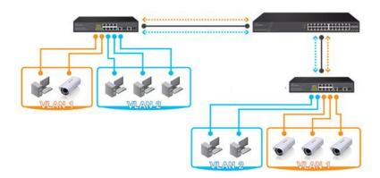
VLANs are most commonly set up using 802.1Q tagging, which adds a header to each frame containing VLAN information. This header is interpreted by the switch and traffic forwarded only to other devices on the same VLAN.
