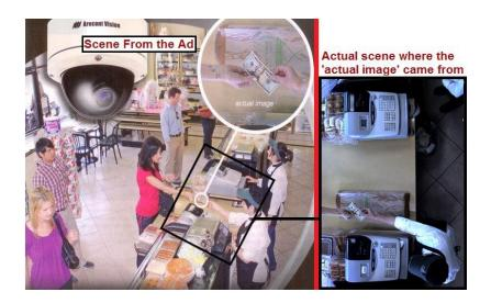
It does not need to be vendor manipulation. Often, people will simply test two different cameras at two different times and not verify that the FoV of the cameras are the same. A wider FoV can result from a shorter lens length or a subject further from the camera. We now examine both.
