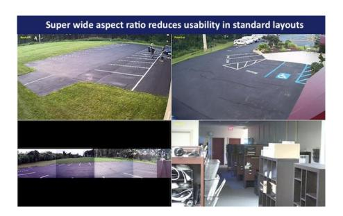
Multi-imager cameras do NOT support any immersive controls nor do they require any dewarping. The video from them is 'flat' like any traditional camera. The only difference is that when the video is 'stitched', it has a far
