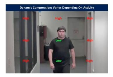
By adjusting compression levels for parts of the scene, it is possible to both reduce overall bandwidth consumed and increased quality in areas which matter by more intelligently assigning compression levels to relevant parts of the scene.
