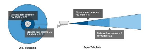
For a 360 / fisheye camera, every 1 foot a subject is further from the camera, the FoV increases ~6 feet (as the FoV is the perimeter of a circle). In just 10 feet, the FoV is more than 60 feet wide.
