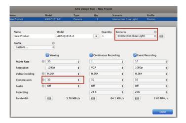
In particular, Axis allows picking from scenes (called scenarios) that adjust projected bandwidth consumption dynamically, e.g., the railway 'station' consumes more bandwidth than the 'stairwell', which is typically with VBR. The image below shows the options and sample videos they provide:
