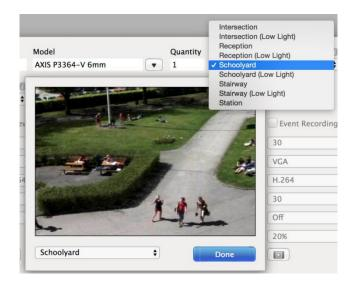
However, even in Axis tool, the choice of scenarios will frequently not reflect one's scenario. For example, there 'intersection' scenario has very little traffic in it and a lot of empty foreground resulting in bandwidth less than the stairwell scenario:
