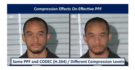
It looks like image B's PPF is far lower than image A, but that is not the case. has far less PPF than image A but that is not the case. Both images are taken from the same camera, with the only difference being increased compression on image B.
