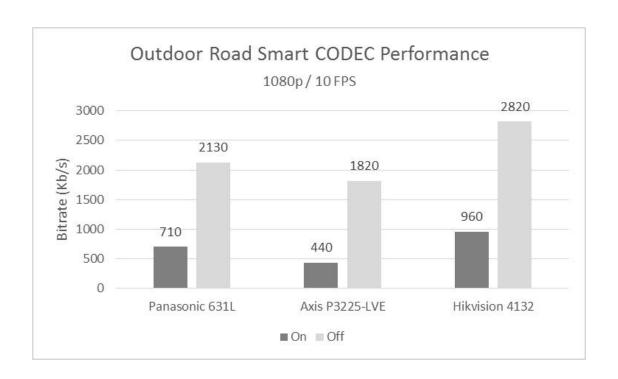
Because smart codecs may have little effect in high motion periods, bandwidth needs must be calculated for worst case bitrates, not average, assuming smart codec savings. Failure to do so could oversaturate and drop wireless or wired links or overload servers.
