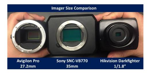
In surveillance, 95% of cameras have imagers that are between 1/2" and 1/4". The most common imager size in surveillance is ~1/3", with 1/2.7" and 1/2.8" common. Previously, lower resolution models (720p/1.3MP and below) often used smaller 1/4" imagers, but even these models predominantly use 1/3" sensors today.
