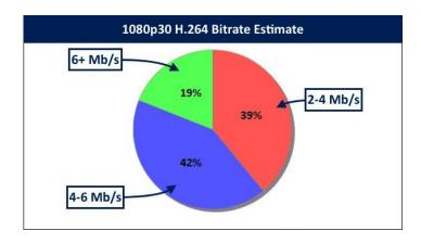
All of the respondents could be 'right' even though the answers vary by more than 300%. Differences in cameras used and sites deployed can easily result in massive differences in actual bandwidth/storage consumed.
