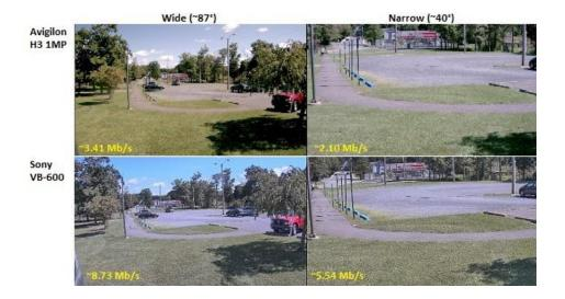
However, in a busy intersection/parking lot, bandwidth decreases by over 50% in the cameras below when widening the field of view. In the narrower FOV, more details of buildings are visible, and the repetitive pattern of the asphalt parking lot may be seen as well, making the scene more difficult to encode.
