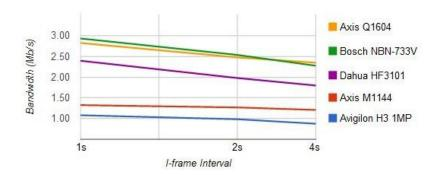
Inversely, increasing the number of I-frames to more than one per second significantly increased bandwidth, despite the minimal increase in image quality.
