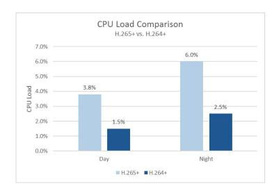
Compounding this issue, while hardware/GPU decoding has become more common in the past several years, many GPUs do not support H.265 hardware decoding. Because of this, while load may be reduced when offloading to the GPU when using H.264, these settings have no effect on H.265 load, shown below:
