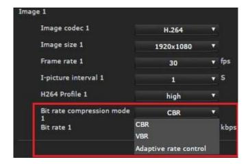
However, note that in Gen 7 cameras (<u>SNC-VM772R</u> and <u>SNC-VB770</u>), <u>Sony</u> does not include any way to fix compression when the camera is set to VBR, instead including only a target bitrate.
