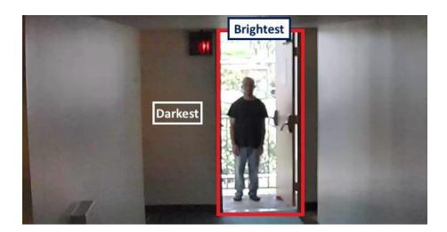
WDR can make a big difference in scenes with widely different light levels. Here's an example of a person walking in a doorway. The non-WDR camera shows only rough details, but not facial recognition, while the true WDR camera clearly shows the subject's face, hairstyle, and more.
