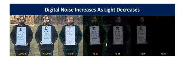
Despite the scene not being 'dark' by typical standards, even the best cameras capture fewer details and display more noise than during the day. However, manufacturer PPF guidelines almost never make this critical limitation clear.
