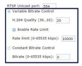
Note that some older versions of Arecont cameras supported only VBR, with no way to cap bitrate and no CBR mode.
