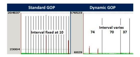
While dynamic I-frame interval will not improve quality, quality should remain essentially the same, while significantly reducing bandwidth. In our tests, dynamic GOP is the largest driver of bandwidth savings in smart codecs.
