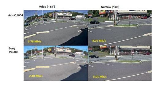
For further details of field of view's impact on bandwidth, see our <u>Advanced Camera Bandwidth Test</u>.
