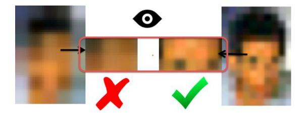
In the former image, the eyes were bigger than the pixels and therefore could not be captured. However, in the latter one, with pixels cover an area smaller than an individual eye, allows the eyes to be captured as two black dots.
