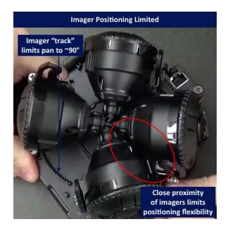
The actual mechanism attaching imagers to the base camera varies as well, with some using a magnetic ring with screw points on it to secure imagers, while others use a fixed track around which imagers slide, shown in examples above.
