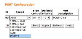
While effective at narrowing the number of potential access points, this step does not necessarily prevent unauthorized access to a network, as someone could potentially unplug a device (camera, workstation, printer) from a previously authorized port or jack and access its port, unless measures such as MAC filtering or 802.1X are in place.
